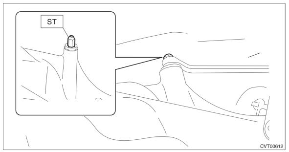
8) Set the ST1, ST2, ST3 and ST4 to the transmission.
