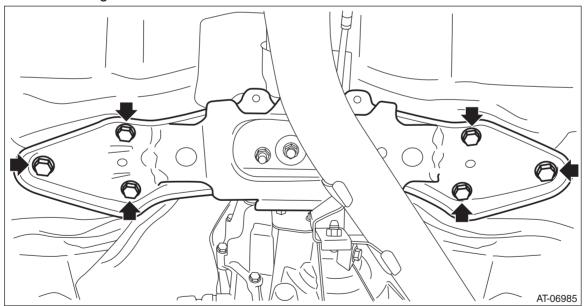
6) Lower the rear side of transmission until the transfer clutch pressure test plug can be removed.
